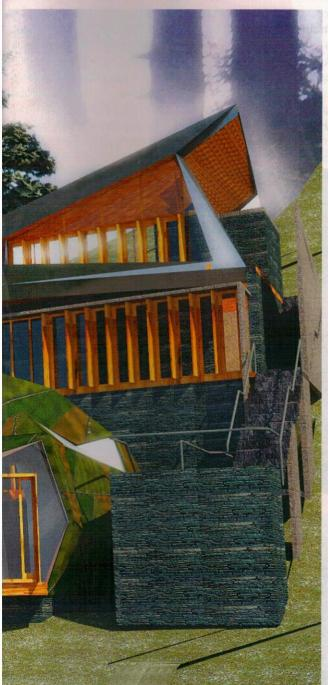
The overall form is envisaged to simulate a cavernous space or an ant hill, sporadically deriving its form from nature. The cottage pods and the roof for the main building have been designed as a composite structure using a skeleton of tubular steel framework covered with thin ferrocement shell. The austere skin of the roof gets a natural makeover by the local flora taking over and imitating like giant moss covered rocks in a forest.
